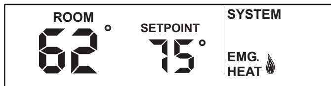
Figure 5. Emergency Heat Mode Enabled
